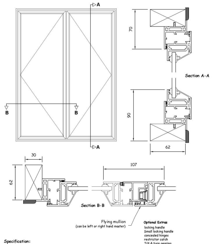
Aluminium 6063T6 alloy to BS EN 755 standard, powder coated to BS 6496 to 60 micron
